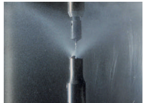
Ultrasonic Atomization of Low Melting Point Alloy and (top left) Gas Atomizer Close Coupled Nozzle
